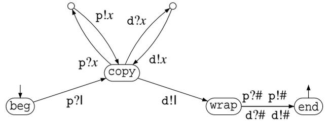
**Figure 2. LCS component that implements rule R1 (assuming purity)**
