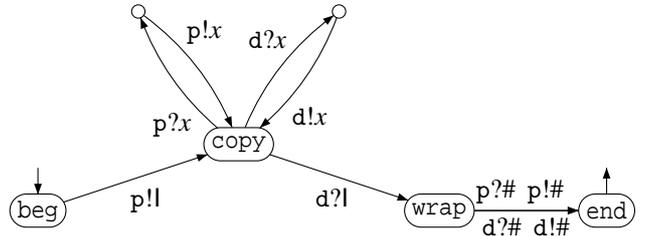
**Figure 5. LCS component that implements rule S1 (assuming purity)**
