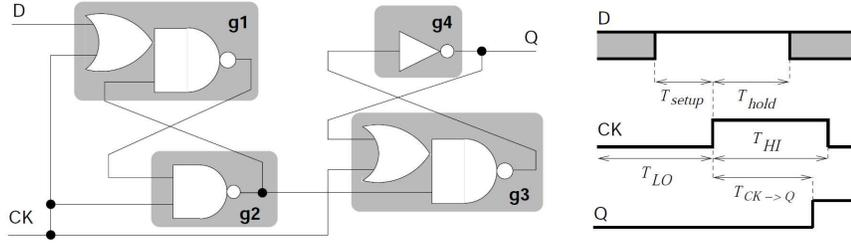
Fig. 2. Flip-flop circuit
